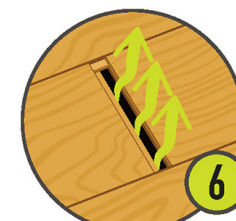
Gaps in suspended floors
