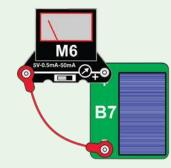
3. Snap wires: Set the meter to the 5V setting and use this circuit to test each snap wire, one at a time. Place the solar cell (B7) near the same light source you used in step 1. The snap wire is damaged if the meter pointer does not move.
