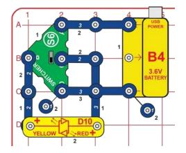
Build the circuit shown. Use the switcher (S6) to control the light.
