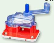
The geared motor (GM) is a motor with a gearbox attached. The crank arm may be attached to it so it can be turned by hand. The gearbox spins the motor shaft faster but with less force than when turning the crank arm.
