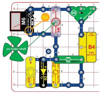
Build the circuit and set the meter (M6) to the 5V setting. Place the wind fan on the motor (M4). Set the switcher (S6) to the left position. The LEDs (D8 & D10) light, the melody IC (U32) makes sound, the fan spins, and the meter shows the voltage across the motor. You may need to give the fan a push to get it started. The voltage produced by the battery is split between the motor and the LEDs and melody IC.
