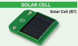
The **solar cell (B7)** contains positively and negatively charged silicon crystals, arranged in layers that cancel each other out. When sunlight shines on it, charged particles in the light unbalance the silicon layers and produce an electrical voltage of up to 7V. The maximum current depends on the type of light and its brightness, but will be much less than a battery can produce. Bright sunlight works best, but incandescent light bulbs also work.
