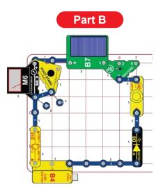
Build the circuit; it has the parts arranged in a loop. Set the meter (M6) to the 0.5mA setting. Set the switcher (S6) to the left position. Place the solar cell (B7) in bright sunlight or near an incandescent lamp. If the light is bright enough, the meter will show a current, the LEDs (D8 & D10) will light, and the melody IC (U32) will make a little noise.
