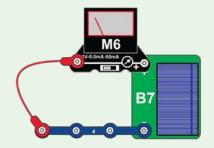
If you prefer, you can test all the snap wires at once using this circuit. If the
