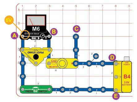
Build the circuit and place the wind fan on the motor (M4). Set the meter (M6) to the 5V setting. Push the press switch (S2); the meter measures the voltage across a resistor in the pivot stand. The measured voltage varies a little as the sound changes.
