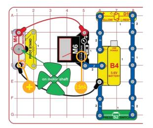
Build the circuit shown. Set the meter (M6) to the 0.5mA setting. Blow hard on the fan or place it in a very strong wind (either outside or near an electric fan). The "windmill" charges the battery (B4) when the wind is blowing hard, and the meter measures the charging current. Push the press switch (S2) to turn on the LED (D10).
