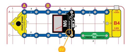
Modify the preceding circuit to be this one, which connects to a different resistor in the pivot stand. Set the meter (M6) to the 5V setting and push the press switch (S2). Read the voltage on the meter.
