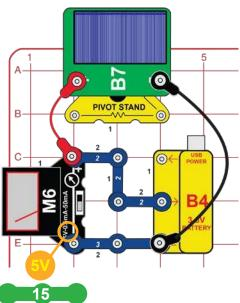
Angle adjustment to light source, measuring charge current:
