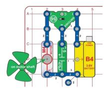
Sometimes motors under a load are difficult to get started. A capacitor can be used to give the motor a little kick. In this project setting the switcher (S6) to the right will charge the 470mF capacitor (C5), then moving it to the left will give the motor a little kick. Since no other power is applied, the motor will not go very far on the small amount of power stored in the capacitor. This is still a good way to get a motor started as power is supplied.
