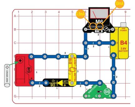
Build the circuit by setting up the parts as shown. Set the meter (M6) to the 0.5mA or 50mA setting. Set the switcher switch (S6) to the right position to connect the rechargeable battery (B4) to the red/yellow LED (D10). If the battery is charged, the LED will light and the meter will show that an electric current is flowing out of the battery. The 0.5mA meter scale will show a high current while the 50mA scale may show little or no current.
