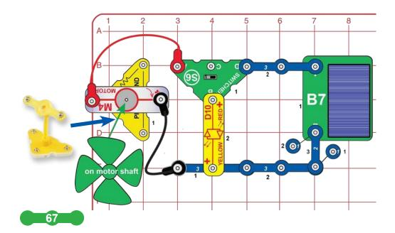
Build the circuit shown, with the motor mounted on the pivot stand like a windmill. Use either sunlight or wind power to run the red/yellow LED (D10). Set the switcher (S6) to the left to use wind power, or to the right to use solar power.
