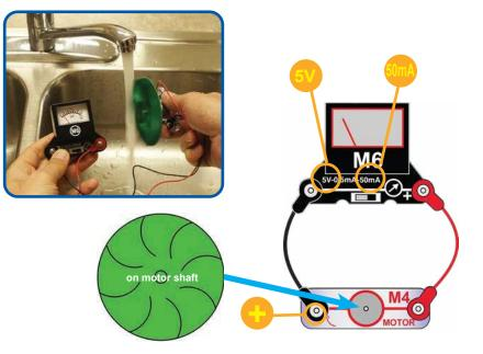
Place the water wheel on the motor (M4) and connect it to the meter (M6), as shown. Set the meter to the 5V or 50mA setting. Hold the motor under a water faucet so the water wheel will "catch" the water as it falls. See how much voltage and current you can produce.
