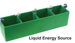
Assemble the liquid energy source using the instructions on page 4. Connect it to the clock (T2) with the red & black jumper wires, the red wire goes to the copper electrode. Fill the compartments with cola soda (other soda flavors and lemon, tomato, or grapefruit juice also work). The clock should be running. Set the time if you like.
