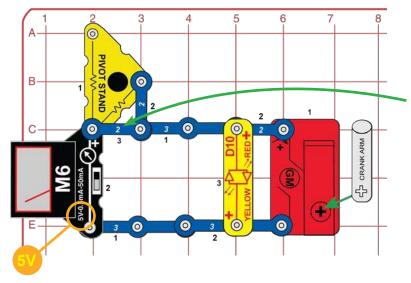
Set the meter (M6) to the 5V setting and turn the crank arm on the geared motor (GM). Turning clockwise will light the red/yellow LED (D10) red while the meter shows the voltage produced. Turning counter-clockwise produces electricity flow in the opposite direction, so the LED lights yellow.
