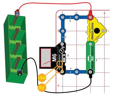
Assemble the liquid energy source using the instructions on page 4. Build the circuit and connect the red & black jumper wires; the red wire goes to the copper electrode. Set the meter (M6) to the 5V setting. Fill the compartments with water. The meter shows the voltage produced, if any.
