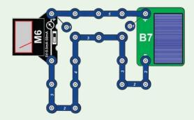
Press switch (S2): Set the meter to the 5V setting and build this circuit. Place the solar cell (B7) near the same light source you used in step 1. If the meter pointer does not move when you press the switch, the switch is damaged.
