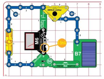
Build the circuit shown. Set the meter (M6) to the 0.5mA setting. Set the switcher (S6) to the right position, place the solar cell (B7) in sunlight or near an incandescent lamp, and push the press switch (S2). The solar cell slowly charges up the 470mF capacitor (C5), and the meter shows the current.
