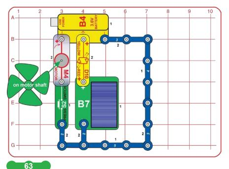
In this project you'll convert one form of energy to another. Place the solar cell in sunlight or about 12 inches from an incandescent light bulb of 60W or more. Adjust the light on the solar cell to make the red/yellow LED (D10) brightest. The solar cell converts light energy into electrical that lights the LED and charges the battery (B4).
