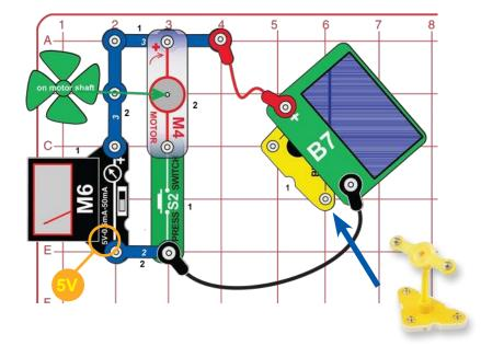
Mount the solar cell (B7) on the pivot stand as shown, and place it in sunlight or near an incandescent lamp. The meter (M6) measures the voltage produced.
