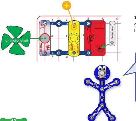
Turn the crank arm clockwise to run the fan and melody IC (U32). Compare how hard it is to turn the crank arm in this circuit and the preceding one.
