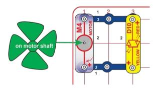
Blow on the fan or spin it with your fingers. The rotating shaft on the motor (M4) generates a current and the LED (D10) lights.
