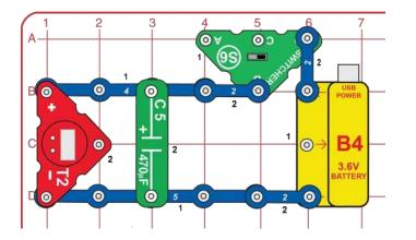
Build the circuit, and set the switcher (S6) to the right position to turn on the clock. If you turn off the switch or disconnect the power source (the B4 battery), the clock will still work for a while. The 470mF capacitor (C5) stores enough electricity to run the clock for a while during power disruptions. If you remove the capacitor, the clock will turn off when you turn off the switch.
