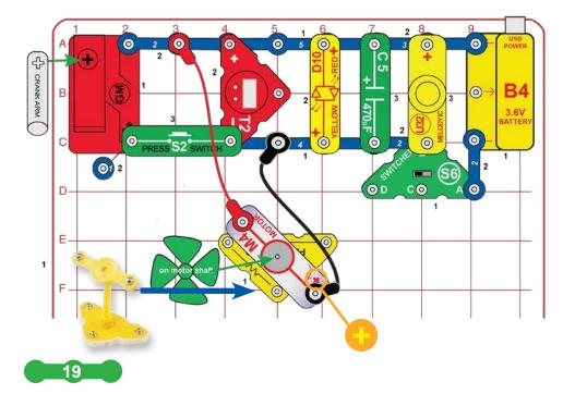
Make sure the battery is charged up (see project 3). Build the circuit with the motor and fan on the pivot stand, and connect the jumper wires as shown. Set the switcher (S6) to the right position to turn on the circuit. The battery runs the clock display (T2), melody IC (U32), red/yellow LED (D10), and windmill (M4). Push the press switch (S2) and the crank arm on the geared motor (GM) will also spin.
