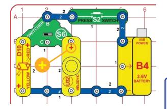
Build the circuit shown and push the press switch (S2) to turn on light or sound. Switches can be arranged in many different ways.
