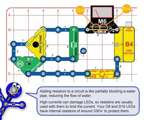
Build the circuit, set the switcher (S6) to the left position, and set the meter (M6) to the 0.5mA setting. This circuit has the red/yellow LED (D10) in series with a 10KW resistor in the pivot stand. 10KW is a high resistance, so the meter measures a small current and the LED is dimly lit. It is easier to see the LED if you take the circuit into a dark room. If the LED does not light at all then the battery needs to be recharged.
