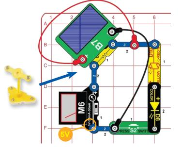
Assemble the pivot, mount the solar cell (B7) on it, and place it in the circuit as shown. Connect the solar cell to the circuit using the red and black jumper wires. Place the circuit so the solar cell is in bright sunlight or close to an incandescent light bulb. Set the meter (M6) to the 5V setting.
