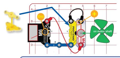
Build the circuit as shown, with the motor (M6) on the pivot and the wind fan on the motor. Set the meter (M6) to the 50mA setting. Blow on the fan or place it in a strong wind.
