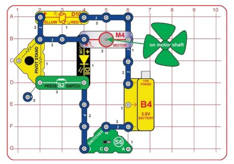
In this circuit we use the LED's (D8 & D10) to indicate if the motor (M4) is spinning. Set the switcher (S6) to the left position, the color LED lights, indicating the motor is not spinning. Pushing the press switch (S2) bypasses the color LED, and it turns off. The voltage across the motor and red/yellow LED increases, so they turn on.
