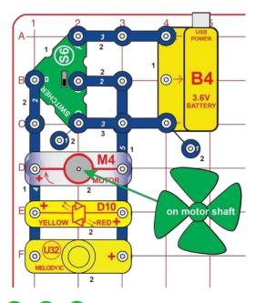
Modify the preceding circuit to be this one. Use the switcher (S6) to control light, sound, and motion. The melody IC (U32) only works in one direction.
