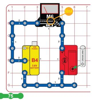
Build the circuit and set the meter (M6) to the 50mA setting. Turn the crank arm on the geared motor (GM) clockwise to charge the battery (B4), the meter measures the current. The battery will be more difficult to charge when it is near full charge.
