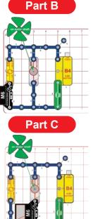
Build the circuit and set the meter (M6) to the 50mA setting. Push the switch (S2); the meter measures the current from the battery (B4). let the fan get to full speed.
