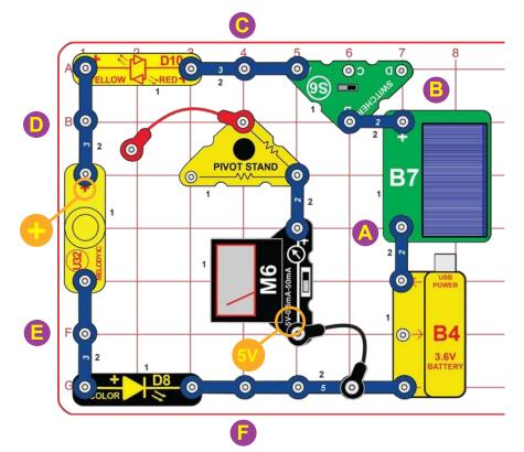
Build the circuit and set the meter (M6) to the 5V setting. Connect the black jumper wire between the meter and 5-snap wire. Connect one end of the red jumper wire to the pivot stand; leave the other end loose. Set the switcher (S6) to the left position. Place the solar cell (B7) in bright sunlight or near an incandescent lamp. If the light is bright enough, the LEDs (D8 & D10) will light and the melody IC will make a little noise.
