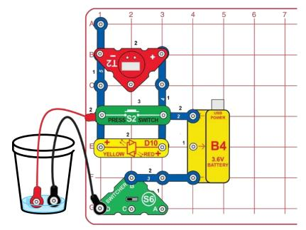
Set the switcher (S6) to the left position. Place the loose ends of the red & black jumper wires into a cup of water without the metal parts touching. The LED (D10) should light dimly and the clock (T2) should run, but it depends on your local water supply. Add salt to the water if they are off or dim to make them brighter.
