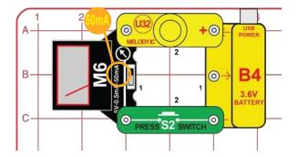
Build the circuit, set the meter (M6) to the 50mA setting. Push the switch (S2) to play a tune on the melody IC (U32), while the meter measures the current through it.
