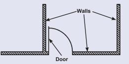
The electronics symbol for a simple switch should be thought of as a door to a circuit, which swings open when the switch is off. The "door" to the circuit is closed when the switch is on. This is shown here:
