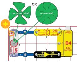
Build the circuit, and place either the wind fan or the water wheel on the motor (M4). To make the LEDs (D8 & D10) bright, blow on the wind fan from above, or blow into the "curves" of the water wheel.
