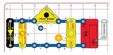
Turn the crank arm on the gearedmotor (GM) slowly clockwise, just enough to turn on the red/yellow LED (D10, which will be red) and make the color LED (D8) show red. Then crank faster, until the color LED also shows green and blue brightly.
