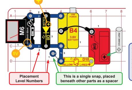
Build the circuit shown here, set the meter (M6) to the 5V setting, and place the crank arm on the geared motor (GM). The meter will measure about 3.6V if the battery is charged up.
