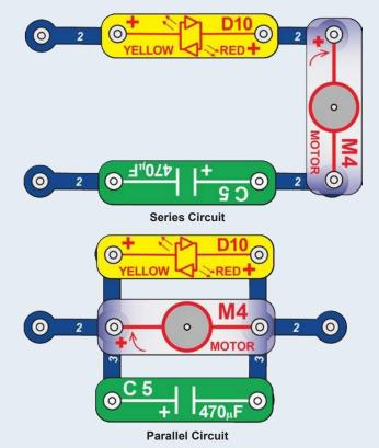
Placing components in series increases the resistance; highest value dominates. Placing components in parallel decreases the resistance; lowest value dominates.
