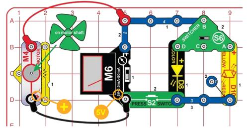
Build the circuit shown. Set the meter to the 5V setting, and the switcher (S6) to the left or right position. Blow on the fan or place it in a strong wind (either outside or near an electric fan). The meter measures how much voltage your "windmill" produces. You may need to give the fan a push to get it started.
