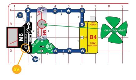
Set meter (M6) to the 5V setting and set the switcher (S6) to the right position. Some of the chemical energy in the battery becomes electricity, which is converted into mechanical energy of motion by the motor (M4).
