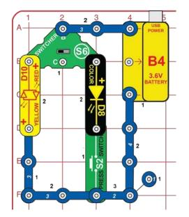
Build the circuit shown. The switcher (S6) and press switch (S2) control the lights.
