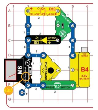
Build the circuit shown. Set the meter (M6) to the 0.5mA setting.
