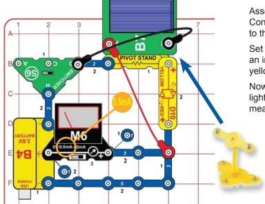
Assemble the pivot, mount the solar cell (B7) on it, and place it in the circuit as shown. Connect the solar cell to the circuit using the red and black jumper wires. Set the meter (M6) to the 0.5mA setting.
