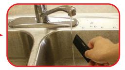
Note: This project works best on a cold dry day. If the weather is humid, the water vapor in the air allows the static electric charge to dissipate, and this project may not work.
