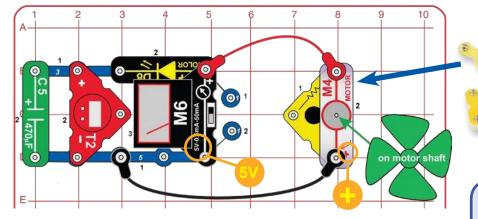
Build the circuit shown. Set the meter to the 5V setting. Blow on the fan or place it in a strong wind (either outside or near an electric fan). The meter (M6) measures how much voltage your "windmill" produces. You may need to give the fan a push to get it started.
