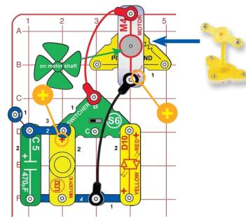
Build the circuit as shown, with the motor on the pivot stand. Set the switcher (S6) to the left for sound (in one wind direction) or to the right for light. Blow on the fan, place it in a strong wind, or give it a good spin with your fingers. The fan must spin very fast to produce sound.
