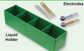
Most sodas and fruit juices are lightly acidic. The acid is similar to the material used in some types of batteries but not nearly as strong. The acid will react with the copper and zinc electrodes to make an electric current, like a battery. Each of the four compartments in the liquid holder produces about 0.7V, but the current is very low and may not last long.
