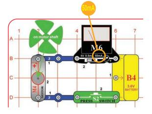
Build the circuit shown. Set the meter (M6) to the 50mA setting and place the wind fan on the motor (M4). Push the press switch (S2) and watch the current on the meter as the motor speeds up.
