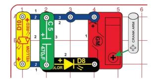
Turn the crank arm clockwise to light the LEDs (D8 & D10). Turn the crank at a constant speed so both LEDs light, and notice how now the red/yellow LED brightness does not vary as much.
