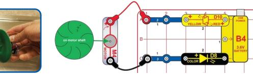
Place the water wheel on the motor (M4) and connect it to the circuit as shown. Hold the motor under a water faucet so the water wheel will "catch" the water as it falls. The LEDs (D8 & D10) should light.
