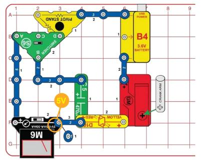
The 470 mF capacitor (C5) is a storage device, so it would be nice to know when it is filled to capacity. With the switcher (S6) in the right position, turn the crank arm until the LED (D10) no longer produces light. When the capacitor is fully charged, the current is blocked and the light cannot turn on.
