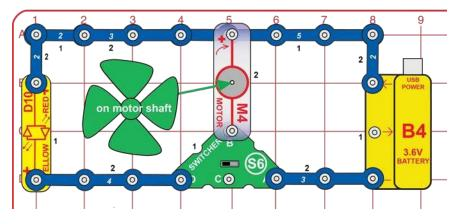
Set the switcher (S6) to the right position. Some of the chemical energy in the battery becomes electricity, which is converted into mechanical energy of motion by the motor (M4).
