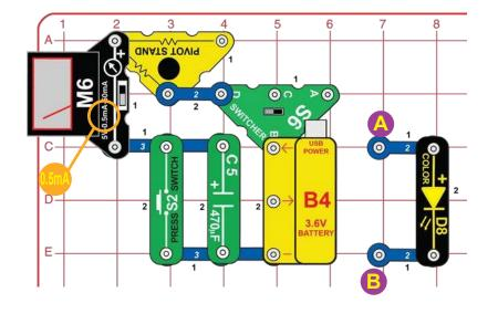
Set the meter (M6) to the 0.5mA setting, and set the switcher (S6) to the left position. Watch the current on the meter as the 470mF capacitor (C5) slowly charges up. Once C5 is near full charge you can push the press switch (S2) to instantly discharge the capacitor and restart the charging process.
