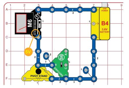
To make a voltage measurement, the meter (M6) is set to 5V and connected in parallel between the two points where the measurement is to be made. Since the voltmeter is in parallel and has a high resistance, very low current flows through it.
