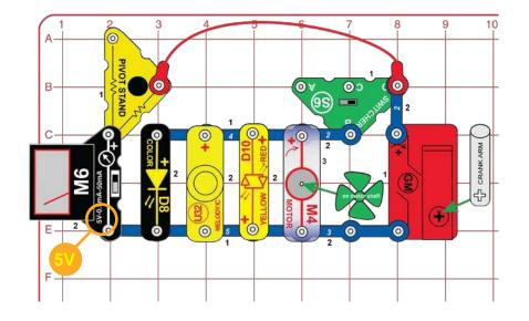
Set the switcher (S6) to the left position, and turn the crank arm. Notice how easy it is to turn the crank, and how high the voltage gets. A resistor in the pivot stand changes the scale to 10V, so double the voltage shown on the meter.
