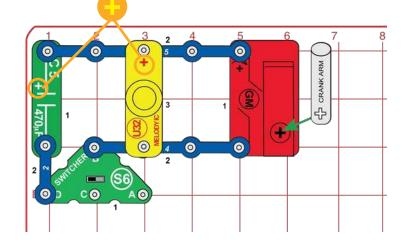
Turn the crank arm on the geared motor (GM) clockwise. The melody IC (U32) makes noise. Set the switcher (S6) to the left position to make the sound a little louder.
