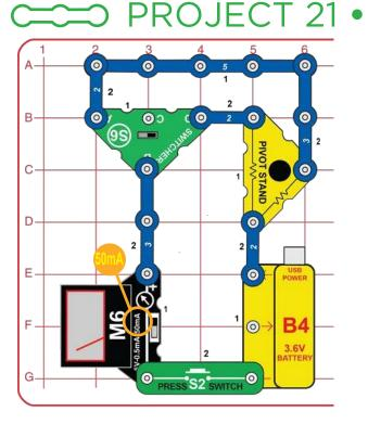
Build the circuit shown. Set the meter (M6) to the 50mA setting and the switcher (S6) to the right position. The pivot stand base has 47W and 10KW resistors in it. They are used to control the flow of electricity in a circuit.
