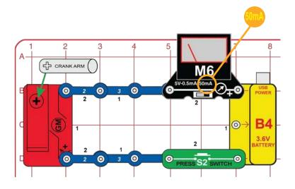
Build the circuit shown. Set the meter (M6) to the 50mA setting. Push the press switch (S2) and watch the current on the meter when the crank arm on the geared motor (GM) spins.
