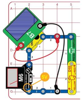
Assemble the pivot, mount the solar cell (B7) on it, and place it in the circuit as shown. Place all the parts with a black 1 next to them on the clear plastic base grid first, then parts marked with a 2. The red/ vellow LED (D10) may be connected in either direction.
