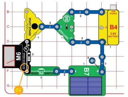
Build the circuit shown. Place the solar cell (B7) in sunlight or close to an incandescent lamp. Set the meter to the 5V setting, but double the reading it shows, since a resistor in the pivot stand converts the scale to 10V. Push the press switch (S2). If the switcher (S6) is set to the upper position, then the meter shows the combined battery (B4) and solar cell (B7) voltage. If it is set to the lower position, then the meter shows only the solar cell voltage.
