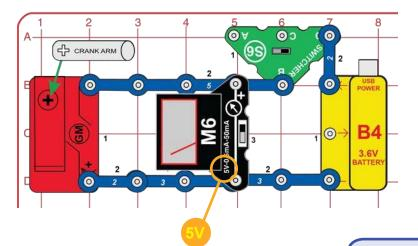
Modify the preceding circuit into this one. Set the meter (M6) to the 5V setting. Set the switcher (S6) to the right position and watch the voltage on the meter when the crank arm spins.
