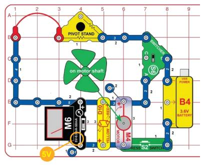
Set the switcher (S6) to the top or bottom position and push the press switch (S2); the motor (M4) spins the fan, the LED (D10) lights, and the meter (M6) measures the voltage across them.
