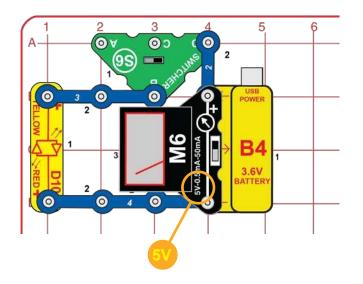
Build the circuit and set the meter (M6) to the 5V setting. Set the switcher (S6) to the right position and watch the voltage on the meter for a while as the battery runs the red/yellow LED (D10). How quickly does the voltage drop?
