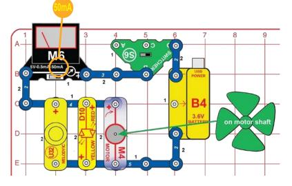
Build the circuit shown. Set the meter to the 50mA setting. Set the switcher (S6) to the right position. The battery operates the melody IC (U32), LED (D10), and motor (M4), just like batteries operate stuff in your home. The meter shows how much current is used to operate them; the more current is used, the faster the battery will run out.
