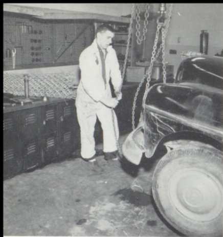
Dave Cornish is lifting Mr. Rice's car in the school shop in order to repair the brakes.
